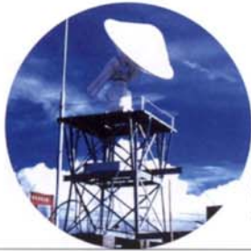
Ground-based 3D Doppler Radar in Tibet for validation of satellite measurements of rainfall
